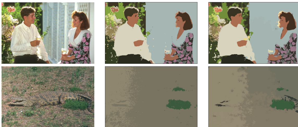
Figure 6. Examples from the Berkeley Segmentation Data Set. Left: Original images. Middle: Original mean shift segmentation. Right: Fast mean shift segmentation. The top row shows a typical example, with RI = 0.91 and GCE = 0.12 . The bottom row shows one of the worst examples, with RI = 0.55 and GCE = 0.15 .
