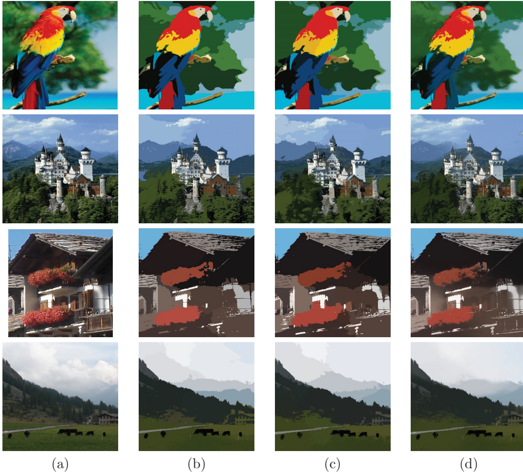
Figure 2. Image segmentation example: (a) the original image, (b) the result of standard mean shift segmentation, (c) the result of fast mean shift segmentation, and (d) the soft segmentation variant of the fast mean shift. Note similar hard segmentation results in (b) and (c).
